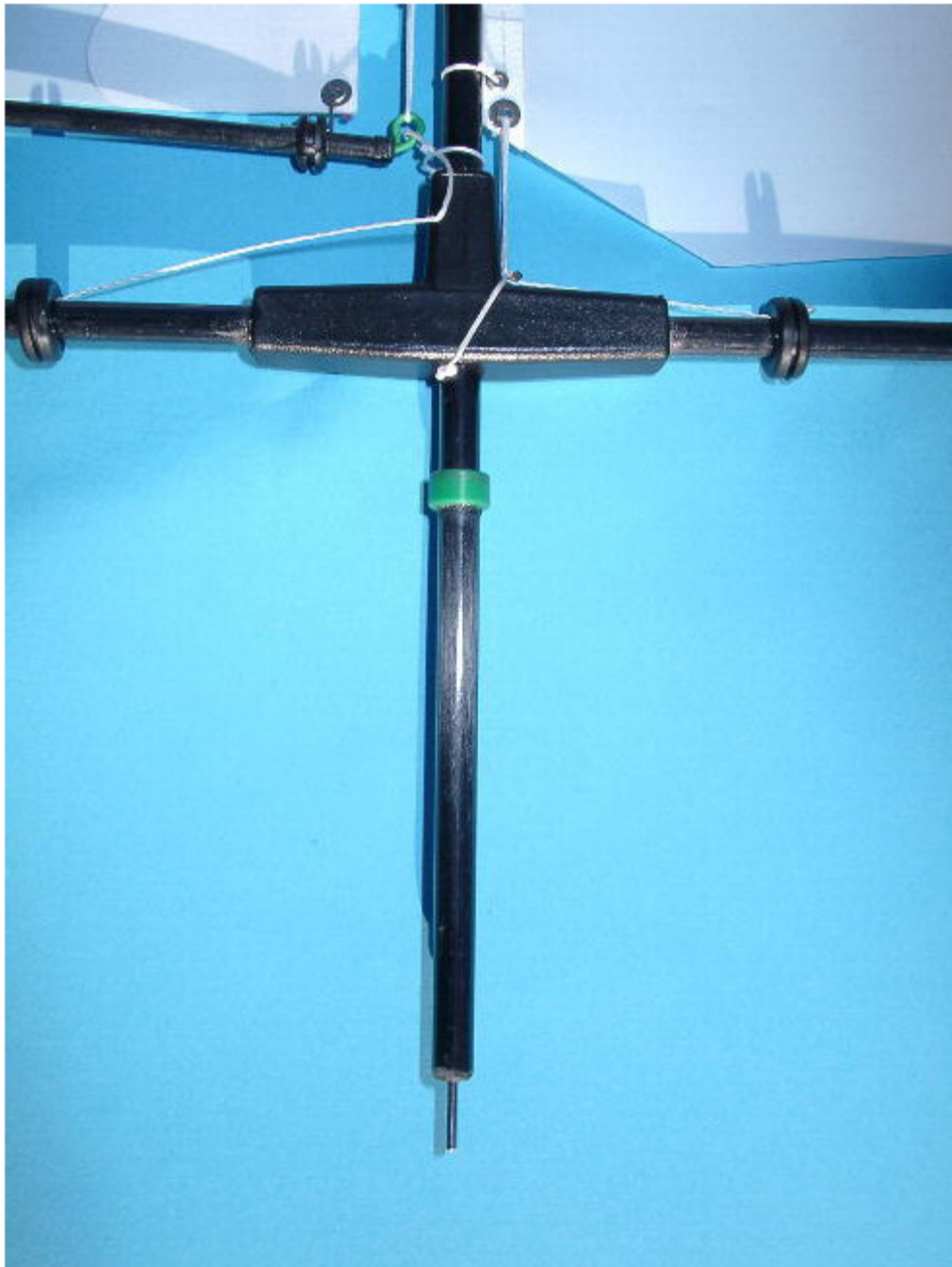
Figure 2: The mast bearings.
