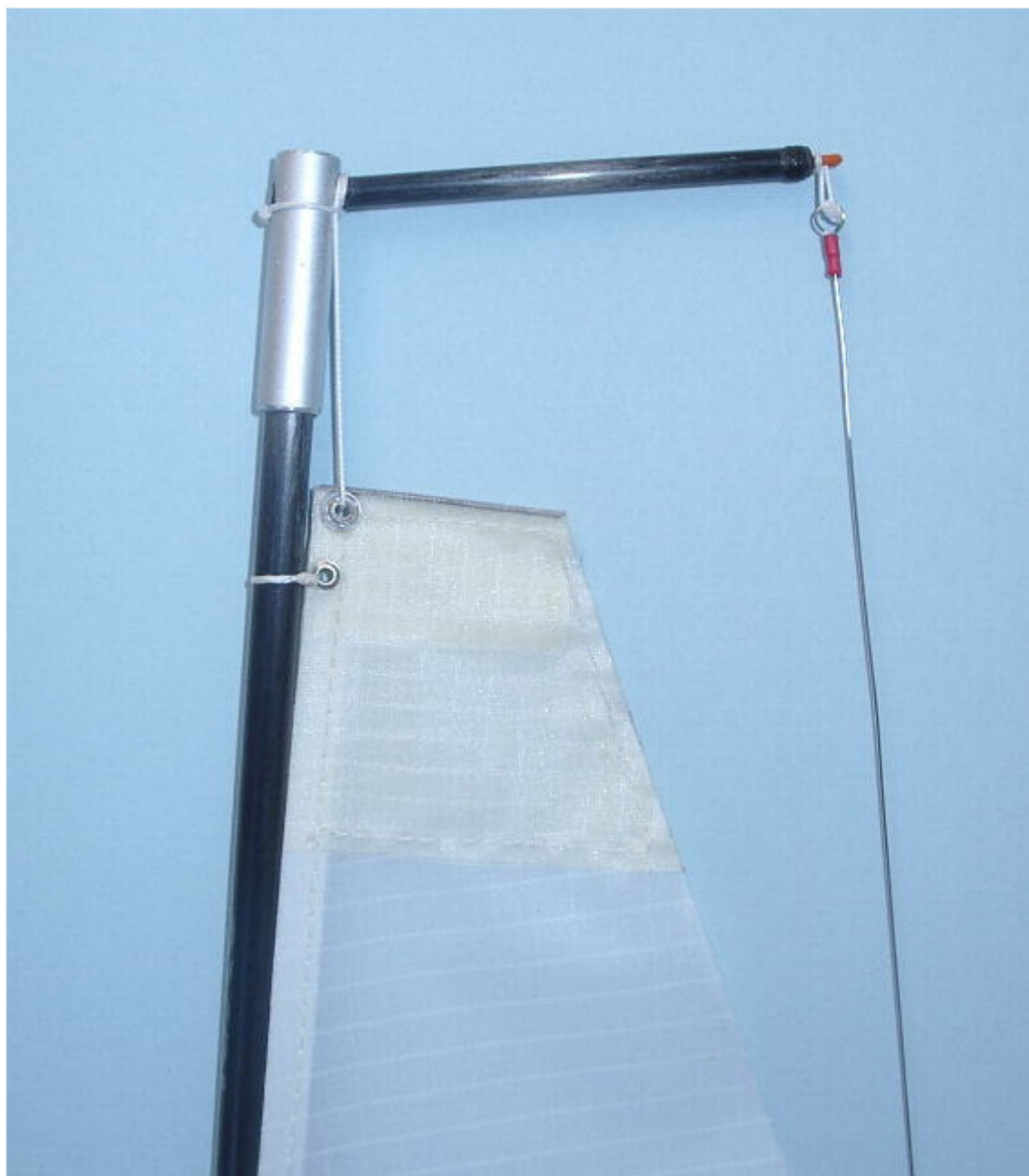
Figure 5: The head of the mainsail with the back stay crane
