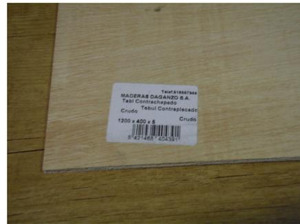
IMAGE 2) Starting Plywood board 1200x400x5 mm
