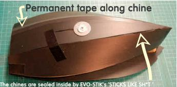
The chines are sealed inside by EVO-STIK's 'STICKS LIKE SH\*T ' (www.bostik.com) as for BUG after the taping outside with jig removed
